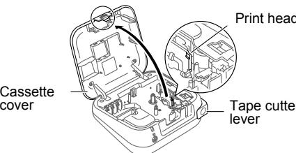
**Open the cassette cover by pressing the above indicated area at the top end of the machine.**
