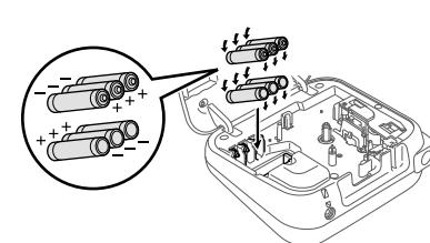
**Insert six new AAA alkaline batteries (LR03) or fully charged Ni-MH batteries (HR03), making sure that their poles point in the correct directions.**
